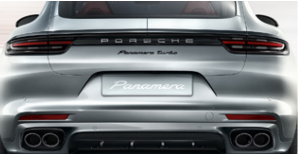
Tinted LED taillights including light strip
