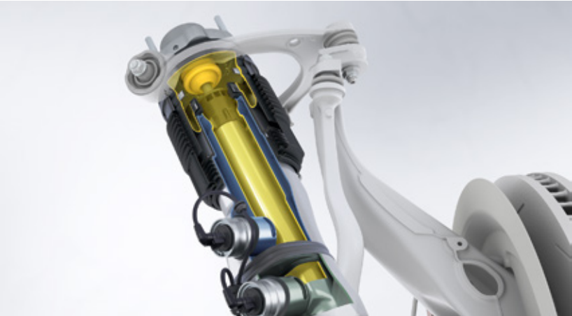
Adaptive air suspension with three-chamber technology
