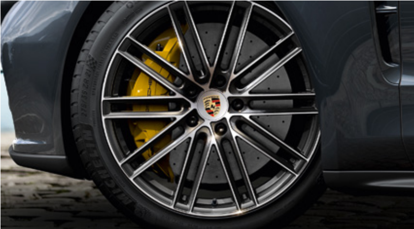
Porsche Ceramic Composite Brake (PCCB)
